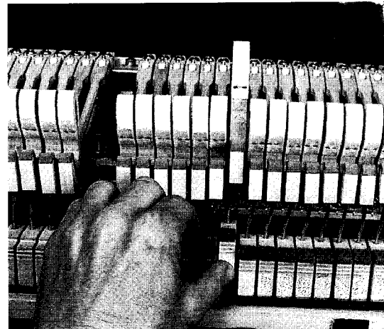
Photo 4 – Observing backcheck alignment: Facing the back of the action, note any backchecks that do not stand vertically; this is easiest to see by focusing on the spaces between neighboring backchecks when at rest. Then, observe side-to-side alignment by lifting the rear of each key, one at a time, to place its hammer in check. Hammer tails are usually tapered, narrower than the backchecks at the bottom and wider at the top, but they should be centered on the backchecks. Ideally, the hammer tails would be shaped square to the shanks and the backchecks adjusted normally.
