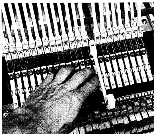
Photo 2 – Checking wippen alignment: Lower one hammer shank at a time over its wippen. Check repetition lever-to-knuckle alignment and clearance between neighboring repetition levers in the drop screw area. Sight down the sides of the wippen to see if the capstan is exposed to either side of the wippen cushion. Most corrections can be made by simply shifting the wippen flange to one side. In this photo, the flange screw is loosened with one hand and the flange is pushed sideways with the screwdriver blade. Then the fingers of the other hand hold the top of the wippen in the new location as the screw is tightened.
